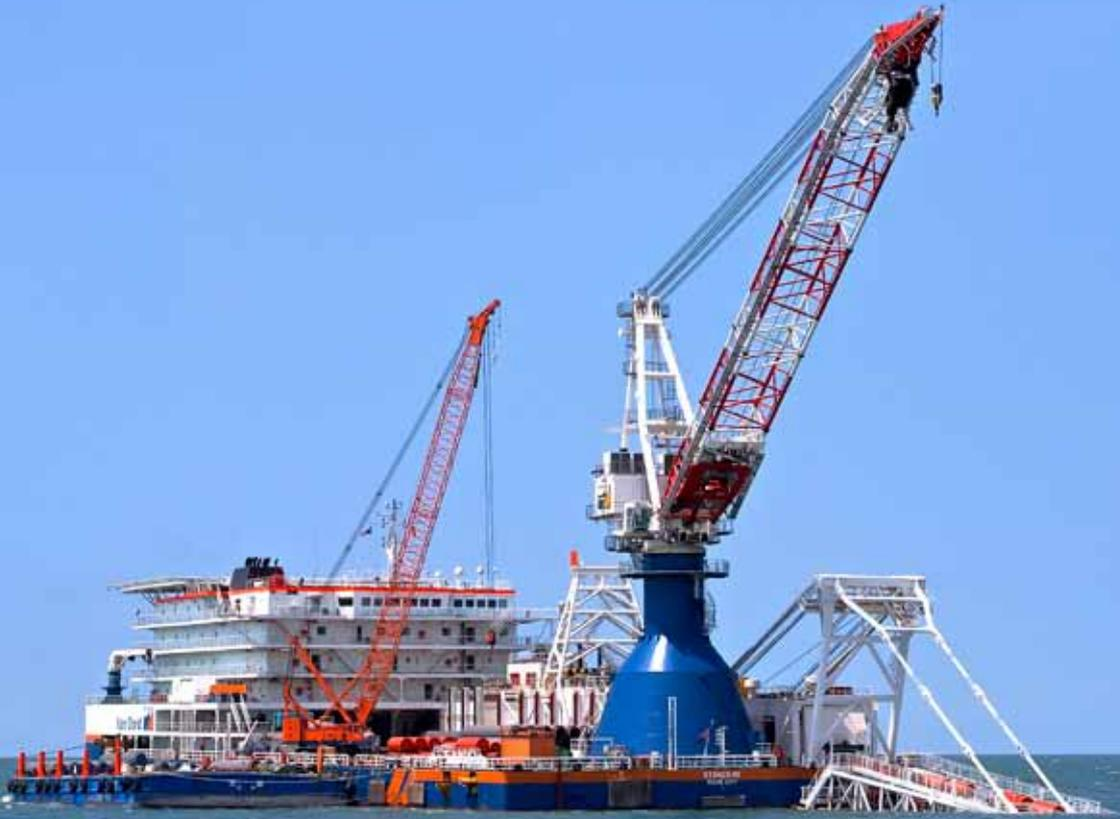
Shallow water pipe lay barge Stingray is equipped with state-of-the-art machinery to install pipelines from 6 to 60 inches in diameter
